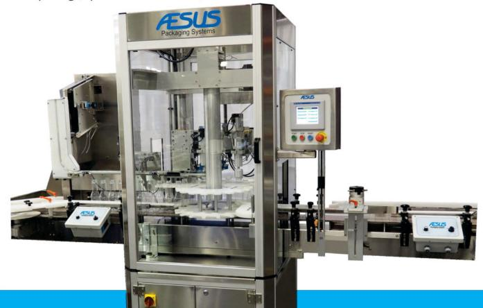
A magnetic clutch will ensure a consistent torque is applied. Easy to operate, the DELTA-Starcapper is ideal for screw caps, child-resistant, pilfer proof and push-on caps and overcaps.
