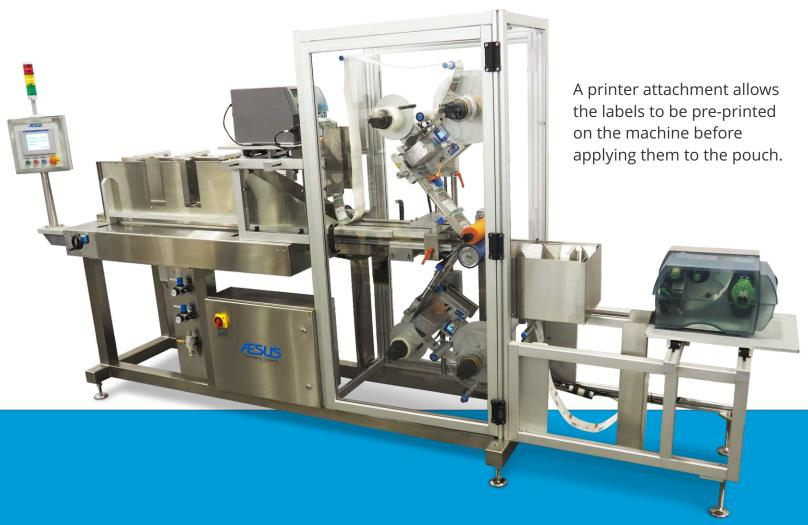
An Exclusive H400 feature is the twist on/twist off Core and rewind holders. Just twist a knob and the core is released to load fresh Labels. The same system for the backing paper. Just the faster label changes will probably pay for your Head! The DeltaPouch also includes a shingled conveyor feeder that provides an autonomy of approximately 5 minutes of operation.
