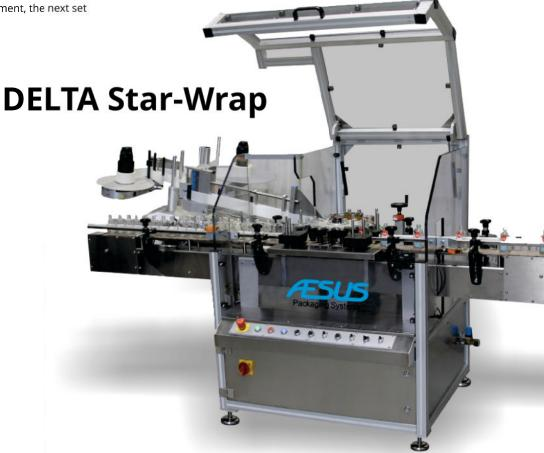
With the same speed and starwheel system as the Premier, the Delta Starwrap is a simpler version without the touch screen, vision systems, verification etc. But it puts on labels just as fast and as accurately.
