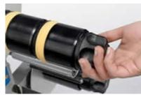
An Exclusive applicator feature is the twist on/twist off Core and rewind holders. Just twist a knob and the core is released to load fresh Labels. The same system for the backing paper.
