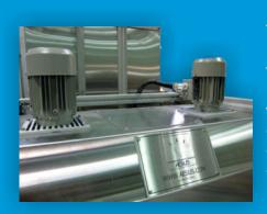
Two air blowers with independent frequency variable speed controls re-circulate hot air within the heat chamber and provides cooling to the outer cabinet.
