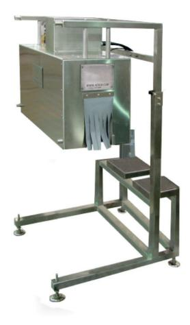
24", 36", 48" or 72" long infra red heat tunnels are ideal for neck banding and full body sleeving, particularly when the containers do not have widely varying contours. Our Tunnels feature one, two or three digital temperature controlled infra red and convection heat zones.
