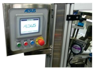
A touch screen HMI (Allen Bradley panel view plus) facilitates easy setup and multiple memories are available to recall setup details. It shows production speeds, and has container and batch counters.
