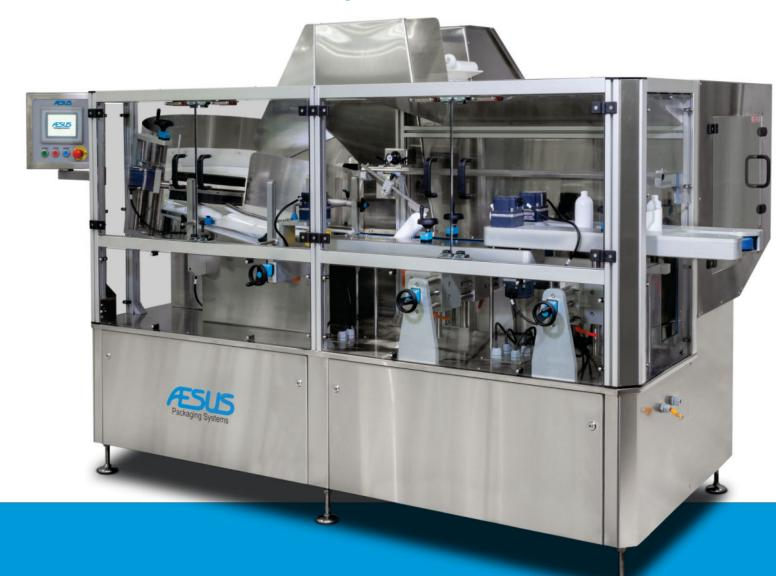
The AesSort bottle unscrambling machine uses the tried and proven hook and belt system that can handle containers from 1 inch diameter through 4 inch diameter and up to 10 inches in height.
