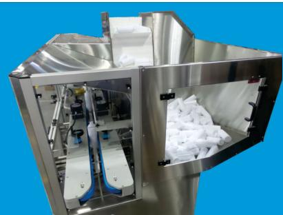
The AesSort is constructed with a heavy duty frame in stainless steel, anodised aluminium, and plastic. The stainless steel Hopper has an interlocked rear door so that the Hopper can be cleaned out or unloaded easily. A typical sensor arrangement is shown; here the sensor controls the level of containers in the sort drum, with a set up scale and easy adjustment knob.
