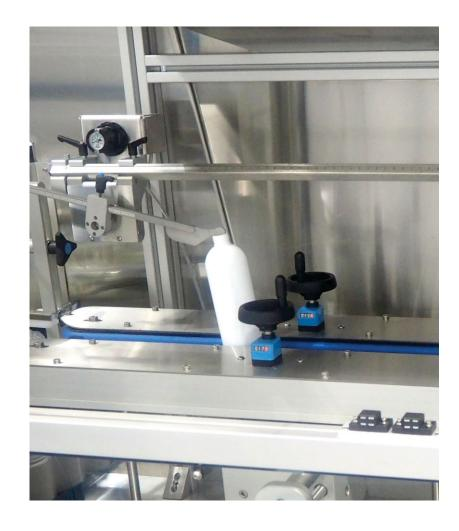
The hook, which inverts containers coming neck first, is unique in that it not only has height adjustment, but the "spring" is controlled by adjustable air pressure as opposed to a fixed spring coil.
